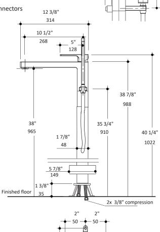
In-floor plumbing connections 2 x 1/2" copper pipe
