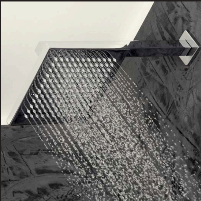
WATERBLADE W1070 shower head W1071 shower arm (shown) Dim.: 8"W 19 1/2"D 4"H Ceiling-mount or wall-mount tilting shower head, 100 easy-clean rubber nozzles, rain flow. Arm with flange sold separately Finish: CR polished chrome, NI brushed nickel
