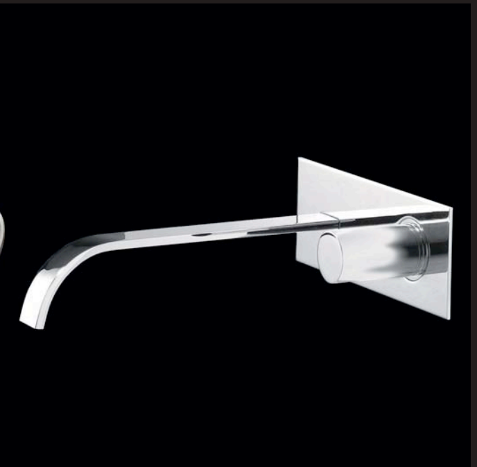
ARCH 13013 faucet Dim.: 8 3/8" SPOUT 4" C/C, backplate 9 1/2" W 3 1/8" H Wall-mount two-hole faucet with one knob handle on the right and backplate, no drain Finish: CR polished chrome
