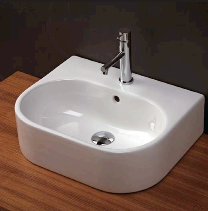
TREVI 2962 lavatory Dim.: 19 3/4"W 15 3/4"D 6"H Wall-mount porcelain lavatory with overflow Options: 01 one faucet hole, 03 three faucet holes in 8" spread 001 white 4207 shroud 4231 pedestal (both shown on opposite page)
