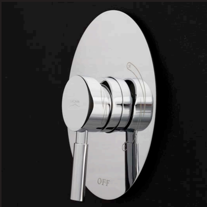
PERLA 0640 mixer Dim.: 5 5/8"W 8 1/8"H Built-in single-lever pressure balancing mixer with oval backplate Finish: CR polished chrome
