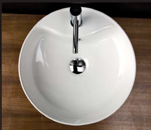
LIGHT CARO 4055 lavatory Dim.: 18 1/4"DIAM 5 3/4"H Vessel porcelain lavatory with overflow Options: 01 one faucet hole 001 white
