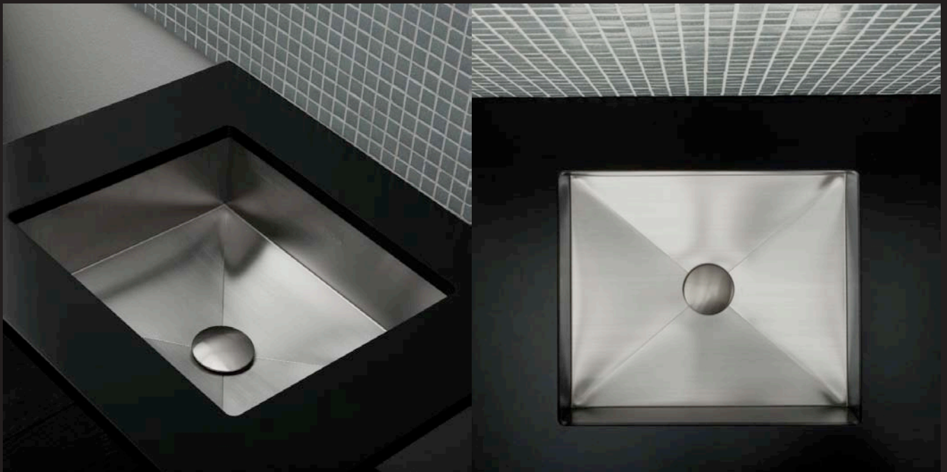
ARGENTO 7400-12 lavatory Dim.: 17"W 14 5/8"D 4 3/4"H Self-rimming or under-counter 16 gauge stainless steel lavatory
