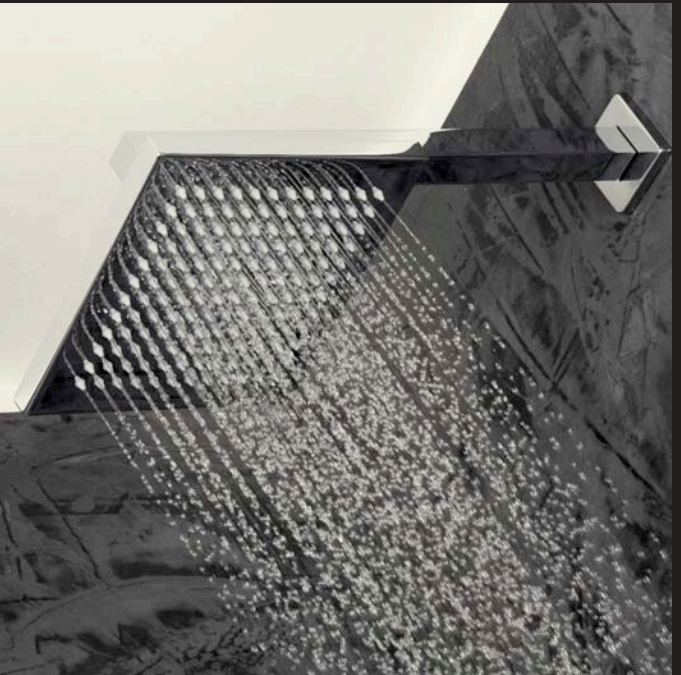
WATERBLADE W1070 shower head W1071 shower arm (shown) Dim.: 8"W 19 1/2"D 4"H Ceiling-mount or wall-mount tilting shower head, 100 easy-clean rubber nozzles, rain flow. Arm with flange sold separately Options: CR polished chrome, NI brushed nickel
