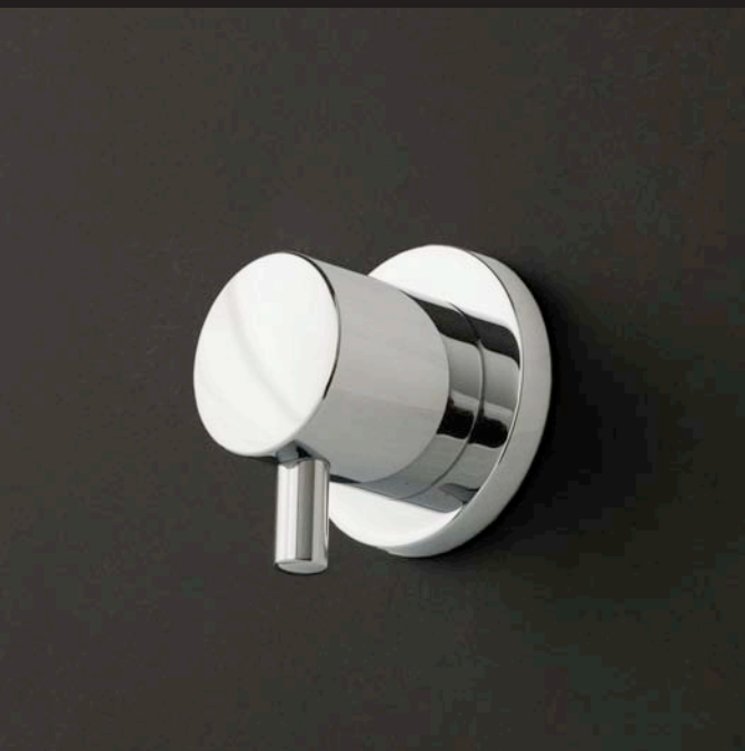
ARCH 260 stop valve Dim.: 2 3/8" DIAM Built-in stop valve with lever handle and round backplate Finish: CR polished chrome Options: 260.5 rough-in 1/2" 260.75 rough-in 3/4"
