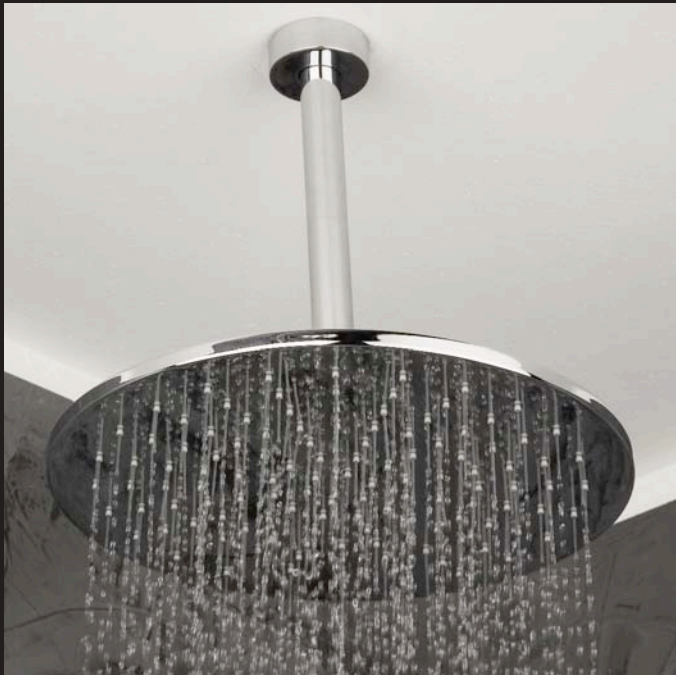
MINIMAL 0426 shower head 0169 shower arm Dim.: 12"DIAM 10"H Ceiling-mount tilting shower head, 126 easy-clean rubber nozzles, rain flow. Arm with flange sold separately Options: CR polished chrome
