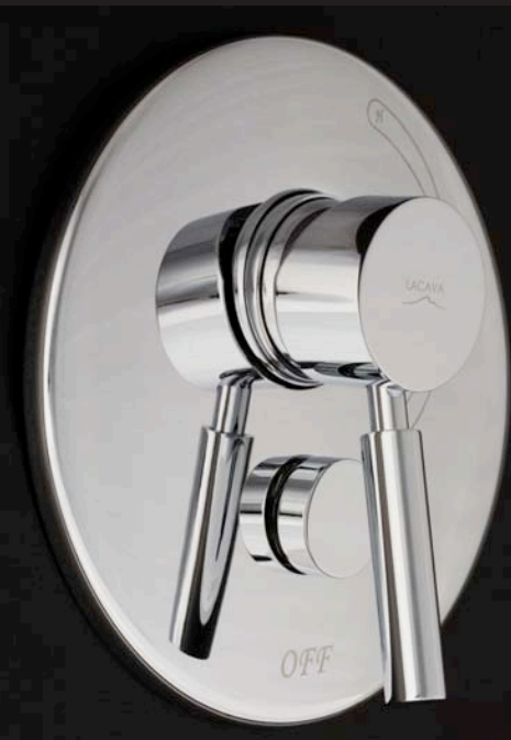
CIGNO 1550 mixer Dim.: 7 1/4" DIAM Built-in single-lever pressure balancing mixer with two-way diverter and round backplate Finish: CR polished chrome
