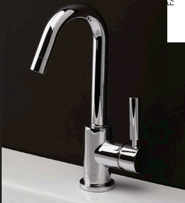
CIGNO 1580 faucet Dim.: 5 1/4" SPOUT 12 1/4"H Deck-mount single-hole faucet with swiveling spout, one lever handle, and a pop-up, drain included Finish: CR polished chrome
