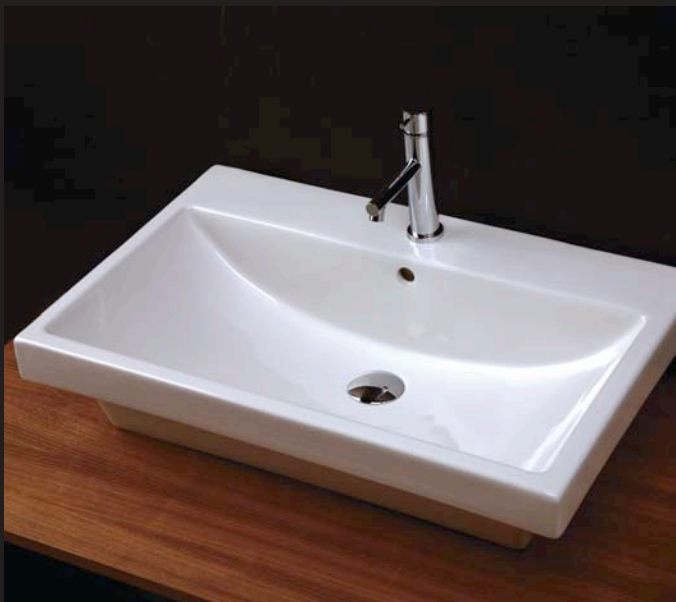
PIAZZA 4271 lavatory Dim.: 27 1/2"W 17 1/2"D 7 1/2"H Wall-mount porcelain lavatory with overflow Options: 01 one faucet hole, 03 three faucet holes in 8" spread 001 white 4207 shroud 4231 pedestal (both shown on opposite page)
