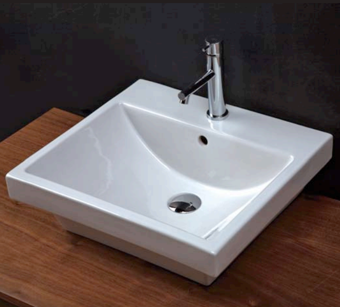
PIAZZA 4272 lavatory Dim.: 19 3/4"W 17 3/4"D 7 1/2"H Wall-mount porcelain lavatory with overflow Options: 01 one faucet hole, 03 three faucet holes in 8" spread 001 white 4207 shroud 4231 pedestal (both shown on opposite page)
