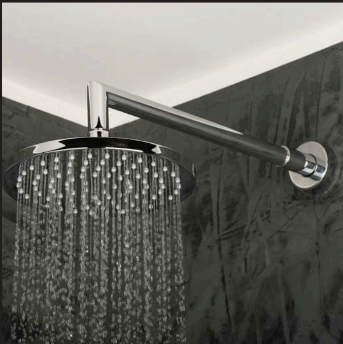
MINIMAL 0416 shower head 0171 shower arm Dim.: 6"DIAM 17 1/2"D 3 1/2"H Wall-mount tilting shower head, 80 easy-clean rubber nozzles, rain flow. Arm with flange sold separately Options: CR polished chrome
