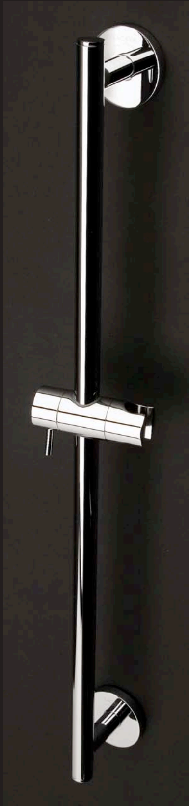
CIGNO 1570 rail Dim.: 2 3/4"D 25 3/4"H Wall-mount round rail with hook for hand-held shower head Finish: CR polished chrome
