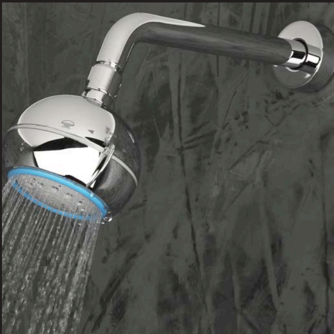
CIGNO 418 shower head 400A shower arm Dim.: 4 3/8"DIA 12 1/2"D 6 1/2"H Wall-mount tilting round shower head, three jets. Arm and flange sold separately Options: CR polished chrome
