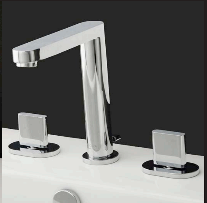
TREVI 2803 faucet Dim.: 5 1/8" SPOUT 6 3/4" H Deck-mount three-hole faucet with a pop-up and spout, two knob handles, and drain included Finish: CR polished chrome
