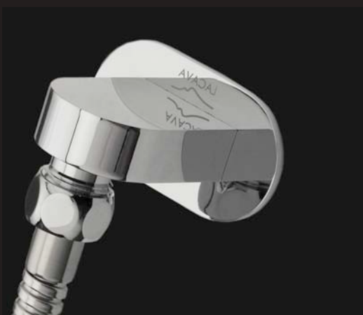
TREVI 2873 water intake Dim.: 2 7/8"W 1 1/2"H Rounded rectangle water intake for hand-held shower head. Hose is not included Finish: CR polished chrome
